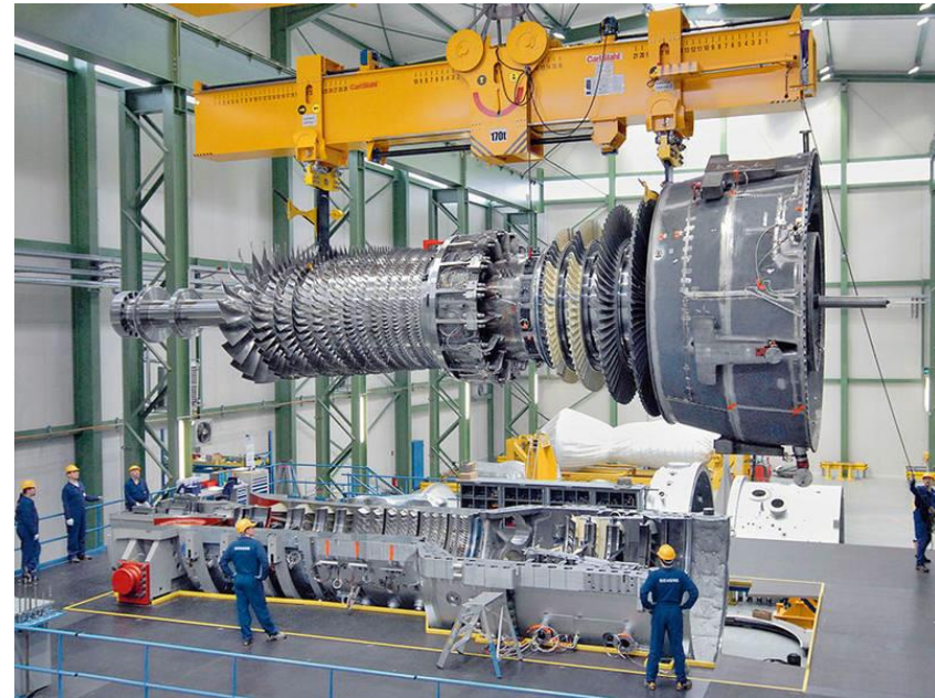
Siemens SGT5-8000H gas turbine (400 MW)
